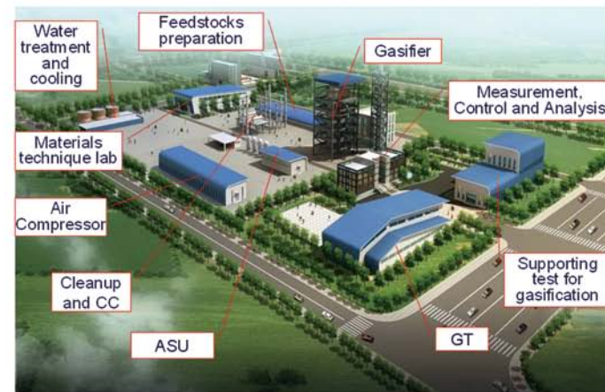
Effect drawing of clean coal energy power system
